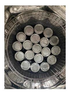
Once sterilization or pasteurization phase is finished, a fast cooling cycle begins, which lowers temperature through a water shower and water immersion system.
