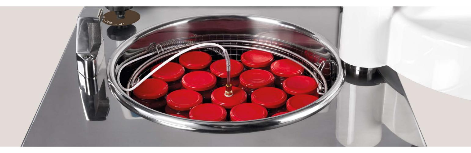
By using a temperature probe placed inside a product sample, we ensure a perfect control of the process, ensuring the correct elimination of all microbial life within each container, while also preserving the organoleptic properties and minimizing possible changes regarding the nutritional value of the packaged product.
