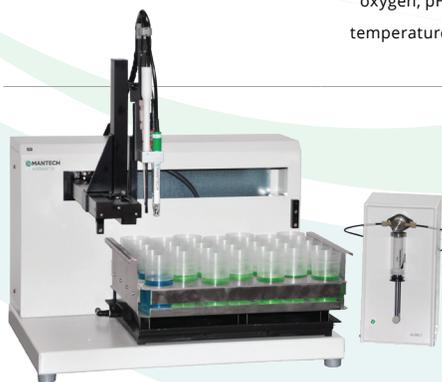
**SYSTEM PICTURED MEASURES PH, CONDUCTIVITY, AND ALKALINITY FROM A SINGLE SAMPLE**
