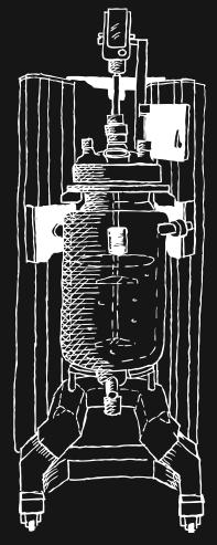
Pilot scale modular jacketed reactor offering multiple setups in one footprint
